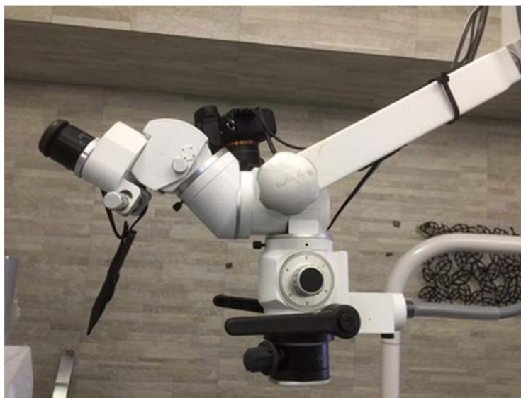
Figure 8.1 Operating microscope showing the binocular, objective, and the nosepiece.
